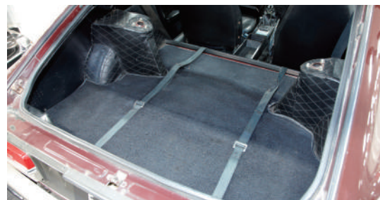
The trunk room was directly connected to the seats, and belts were provided to secure luggage.
