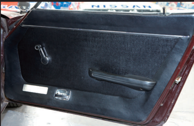
The door interior opening and closing lever is positioned quite low. This is designed to match the seating position.
