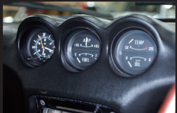
The trio of gauges from left to right includes the clock, ammeter & fuel gauge, and water temperature & oil pressure gauge. This three-gauge setup has also been carried over to the current Fairlady Z.
