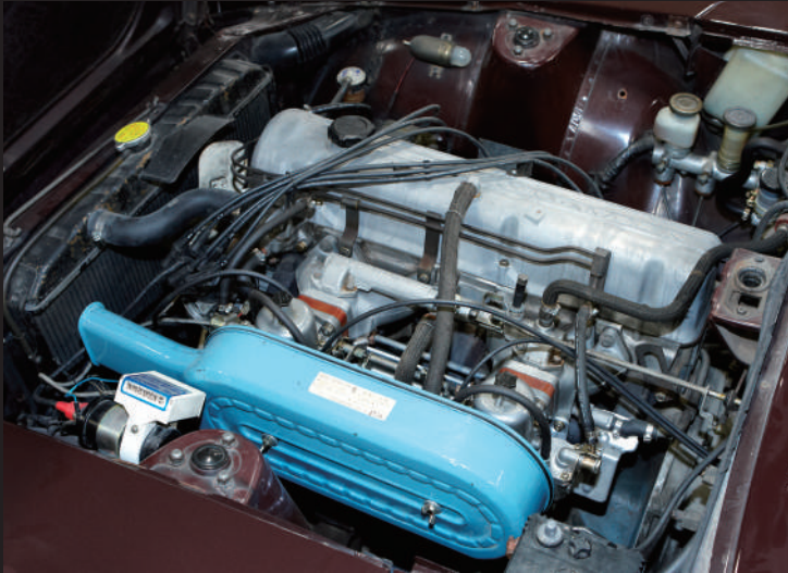
The L24 engine, with intake and exhaust valves aligned on one side, features a layout where both the carburetor and exhaust pipe are positioned on the same side.
