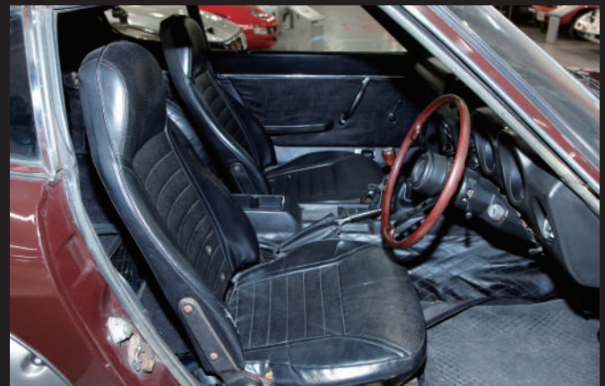
High-back seats with integrated headrests. They feature a reclining function, allowing for a stable driving position.
