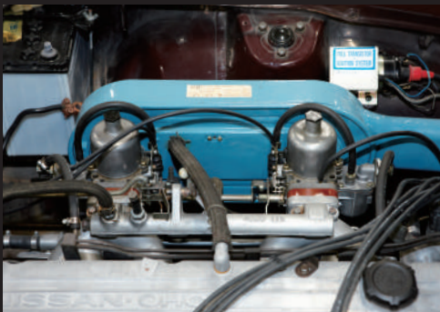
Two carburetors, enlarged from 38mm to 46mm to match the increased engine displacement, were installed.
