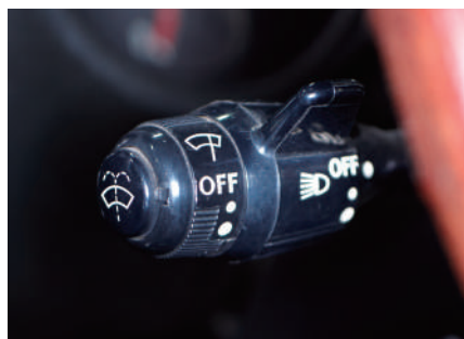
The switches for lights, wipers, and other controls were integrated to the left side of the steering wheel for improved operability.
